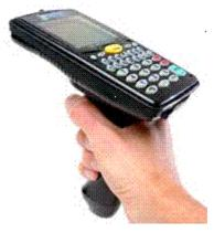
Use of the optional Portable Bar Code Reader (*left*) with Archive Manager is simple and practical, and provides tremendous savings as compared to collecting data manually. Archive Manager downloads the collected data from the reader to a text file on the host PC as ASCII characters (unformatted text). A guide to the data format used in these files in located in *Appendix B* of this manual.
